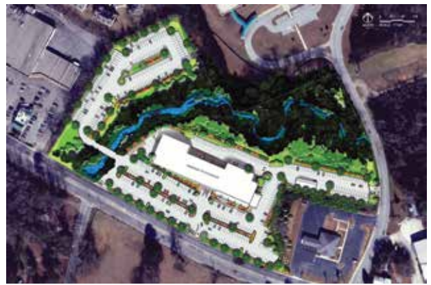
The overall site plan. The creek that bisects the site required buffering in accordance with Lexington County regulations.
