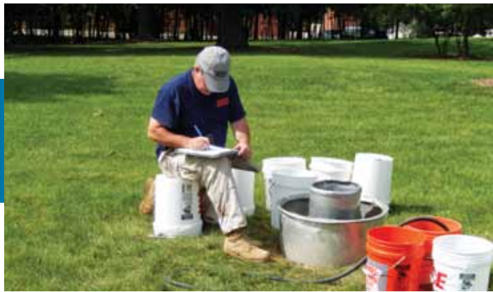
A worker prepares to insert the double-ring infiltration equipment per ASTM 3385 as modified by the Wisconsin Department of Natural Resources for grass bioswales.
