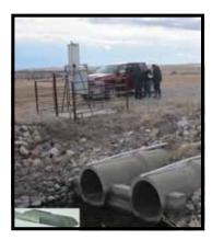
**Stormwater Flow Meters Measure Flow in Open Pipes and Channels**
