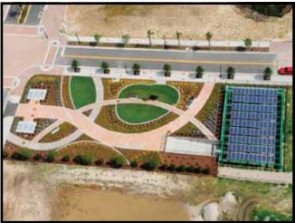
walkways. Permeable pavers were used for the center median of the main thoroughfare to reduce the heat island effect and aid in storm water management.
