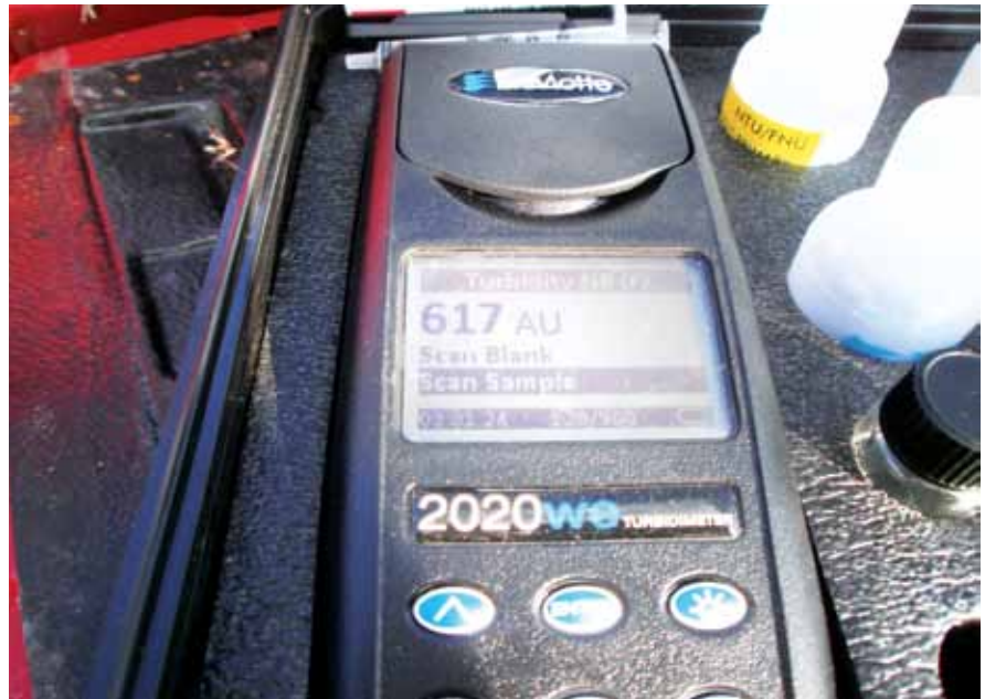
The initial turbidity of the storm water canals lining the Tampa International Airport was 617—almost 20 times higher than required by state regulations.
