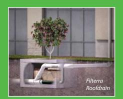
This new design tested at Colorado State University Hydraulics Laboratory treats roof or other **piped in** runoff and also eliminates the need for additional overflow structures.
