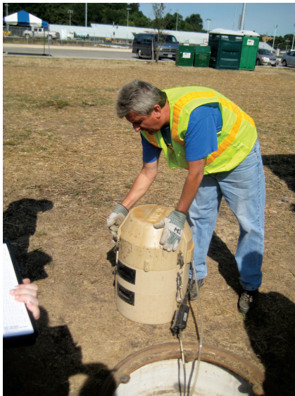
MMSD staff members take samples representing the first and second flush from storm sewers. Top right: Samples are tested for 30 contaminants and sent to GLWI for further analysis.
