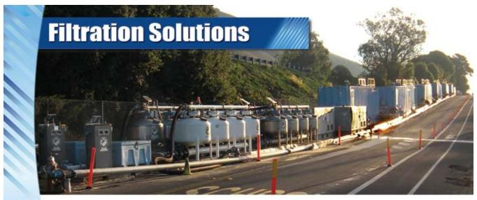
**Challenge:** Filter water from pigged pipelines from over 18,000 to 225 NTU.
